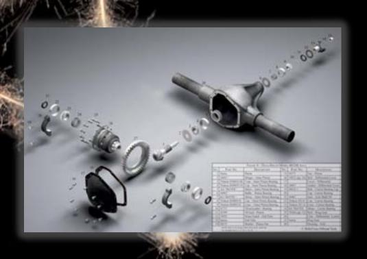
Feature-based CAD constructs designs from smaller, interdependent parts
